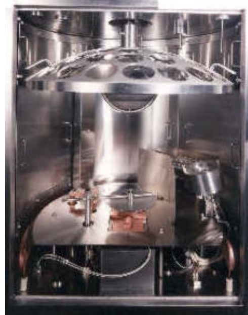
Figure 5: Domed calotte, electron beam gun and ion source are visible in this ophthalmic coater.
